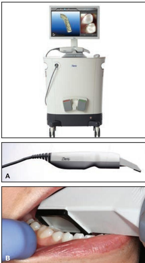
**Fig. 5 A.** iTero intraoral scanner with sealed keyboard, wireless mouse, and wireless foot pedal; parallel confocal imaging enables powder-free scanning. **B.** Wand held at 45° to capture both lingual and occlusal surfaces.
