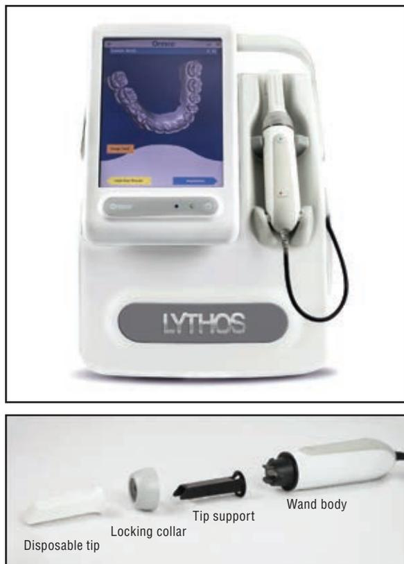
**Fig. 7 Lythos intraoral scanner featuring compact design and touchscreen monitor with extension arm; accordion fringe interferometry enables powder-free scanning at video speed.**
